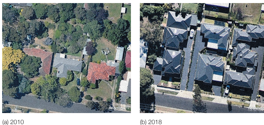
Figure 13: Redevelopment of (a) three allotments with three detached dwellings, to yield (b) eight dwellings (Source: Nearmap).
