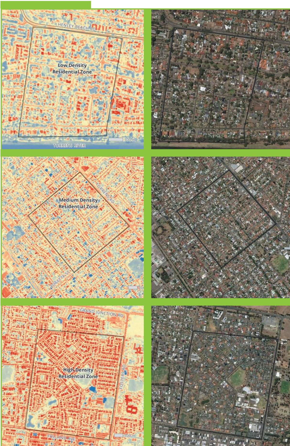
Figure 12: Surface temperature differences in low (Fulham), medium (West Croydon), and high (Northgate) density residential zones (Source: Western Adelaide Urban Heat Mapping Project Report)
